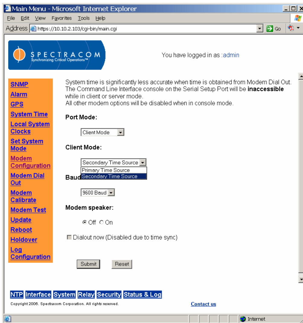
Figure 7-2: System Modem Configuration Screen, Client Mode
